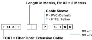
XX = ST, Metal Connector (Default) XX = DC, Dielectric Connector at one end
